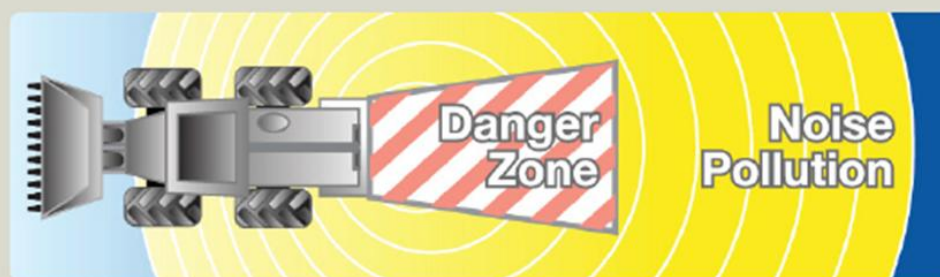
Broadband alarms generate warning noise in the danger zone but less spilled noise than tonal alarms
