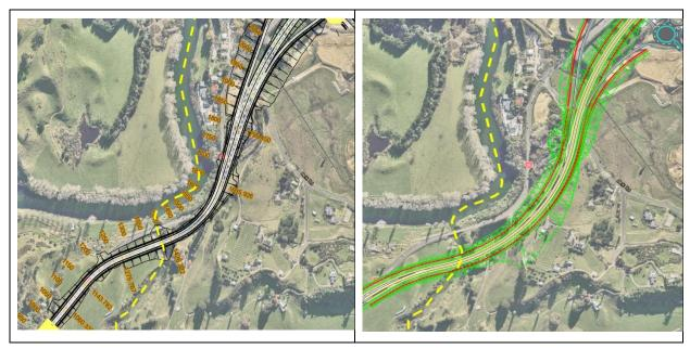
Figure 4-5. Omanawa Stream Alignment – Difference between Option 2 (left) and Hybrid Option 2 (right)
