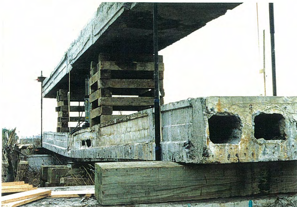
Figure 7. Test just before failure in the second cycle. Note significant sag in test beam.
