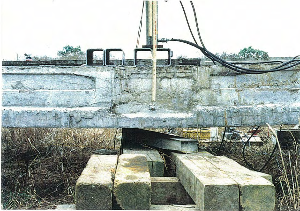
Figure 7. Test just before failure in the second cycle. Note significant sag in test beam.
