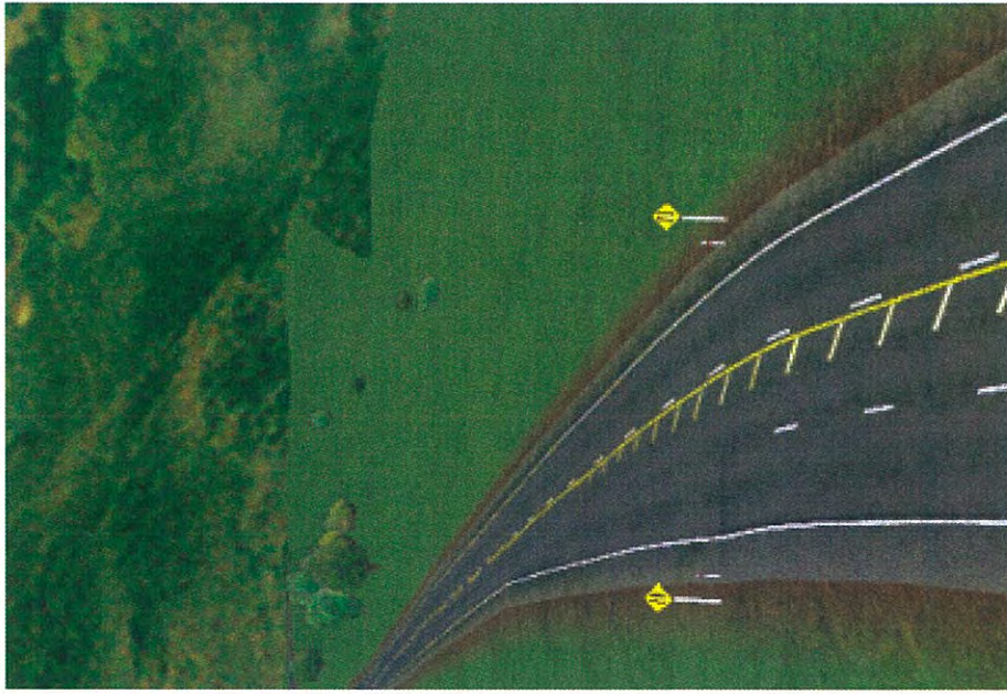
Figure 5.30 Oblique scan (left) and screen shot of plan view (right) of the simulated right herringbone with short taper merge design.
