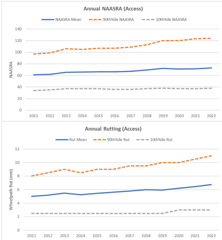
Figure 8-1 Roughness & Rutting Progression for Access Highways
