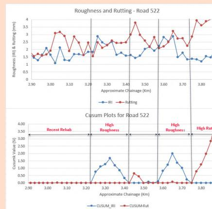
**A treatment length is a uniformly performing contiguous section of road, and performing differently from the adjacent sections**
