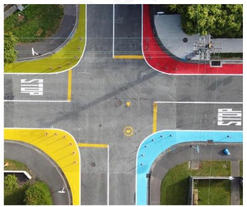
Figure 9: delineator posts and paint tighten corners (Nelson City Council)
