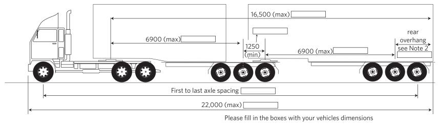
**Note 1** Tractor can be 3-axle or 4-axle with twin steer
