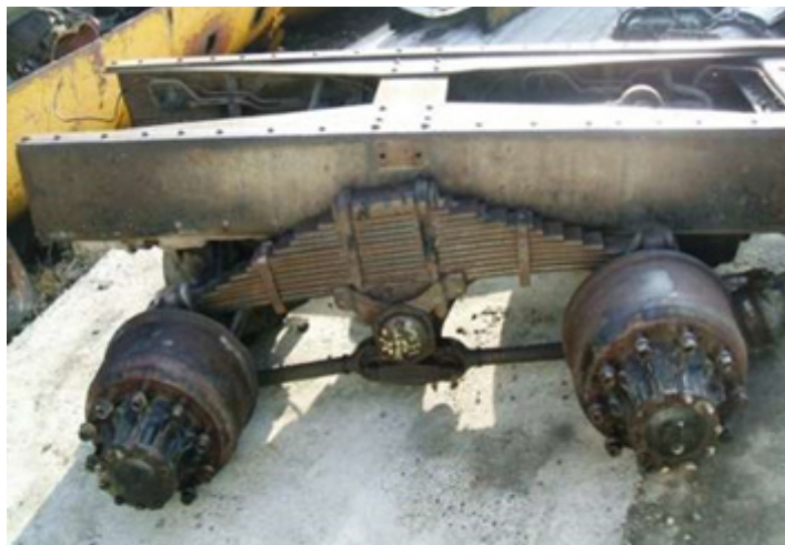
Figure 3: A typical tandem axle trunnion type rear suspension system (source NZ Police)
