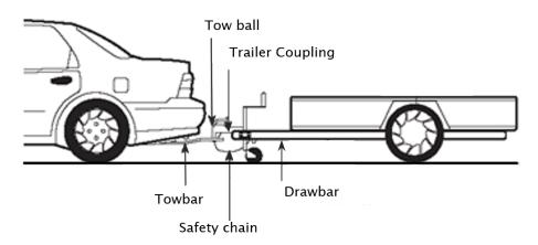
Diagram showing the parts of a trailer
