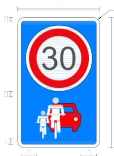
4. The required sign for waste collection trucks to comply with TMP requirements will be the RD-6R variant. Ideally the sign would be hinged or active to be able to be used only when the truck was actively blocking a cyclist lane or engaged in waste collection.
