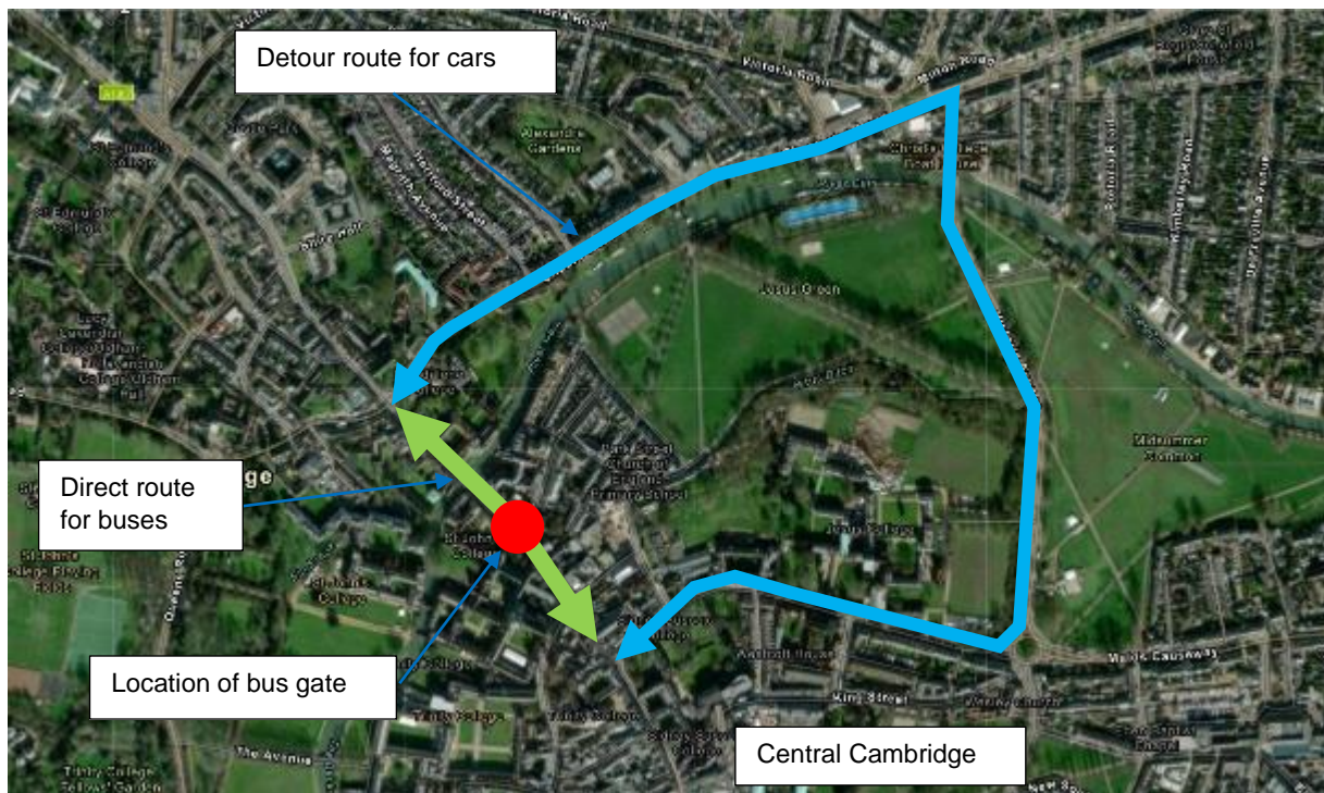
Figure 61 – Comparison of the route for buses and cars resulting from the Bridge Street bus gate in Cambridge, United Kingdom. Source: Esri.
