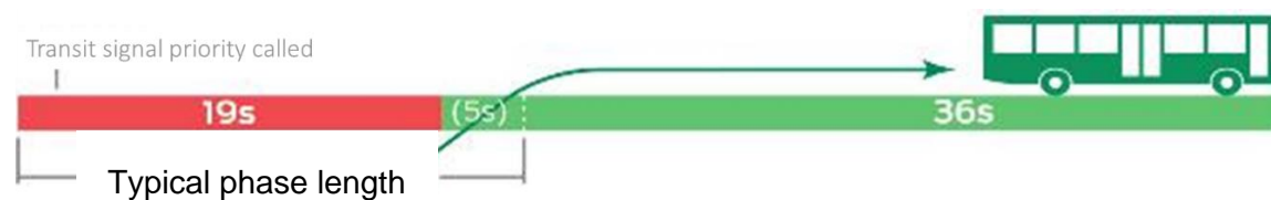
Figure 45 – Red truncation in signal phasing (s = seconds). Source: National Association of City Transportation Officials. No date. Active transit signal priority in Transit Street Design Guide .
