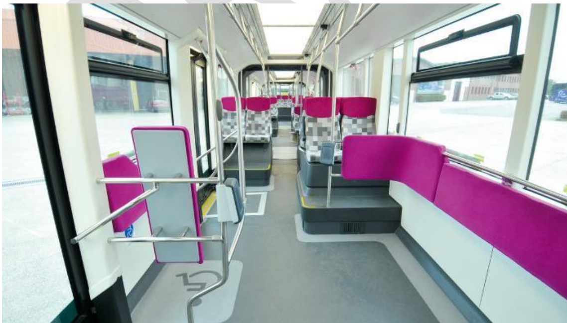
Figure 65 – Interior of a bus optimised for standing room with a standing area and wheelchair space near the door and standard seats placed away from the door. Source: Van Hool.
