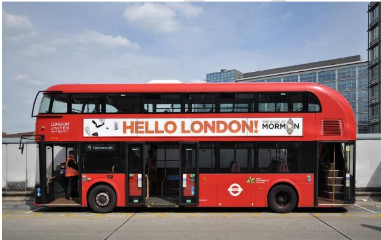
Figure 71 – London Routemaster, which is double-deck bus with three sets of doors and two sets of stairs. Source: Ron Ellis.
