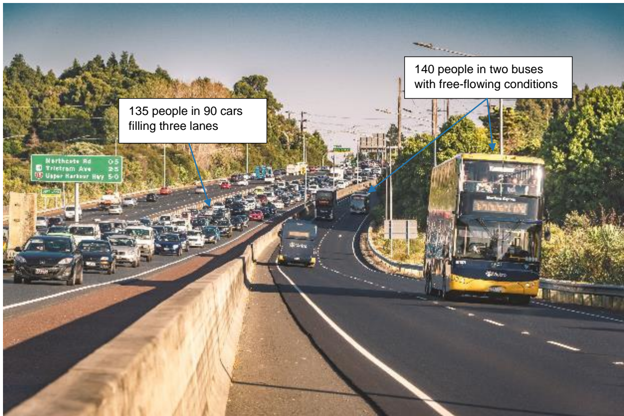
Figure 79 – Number of people in three full traffic lanes with one busway lane (assumes average car occupancy of 1.5 people per vehicle and 70 passengers per bus), Auckland Northern Motorway. Source: Auckland Transport.
