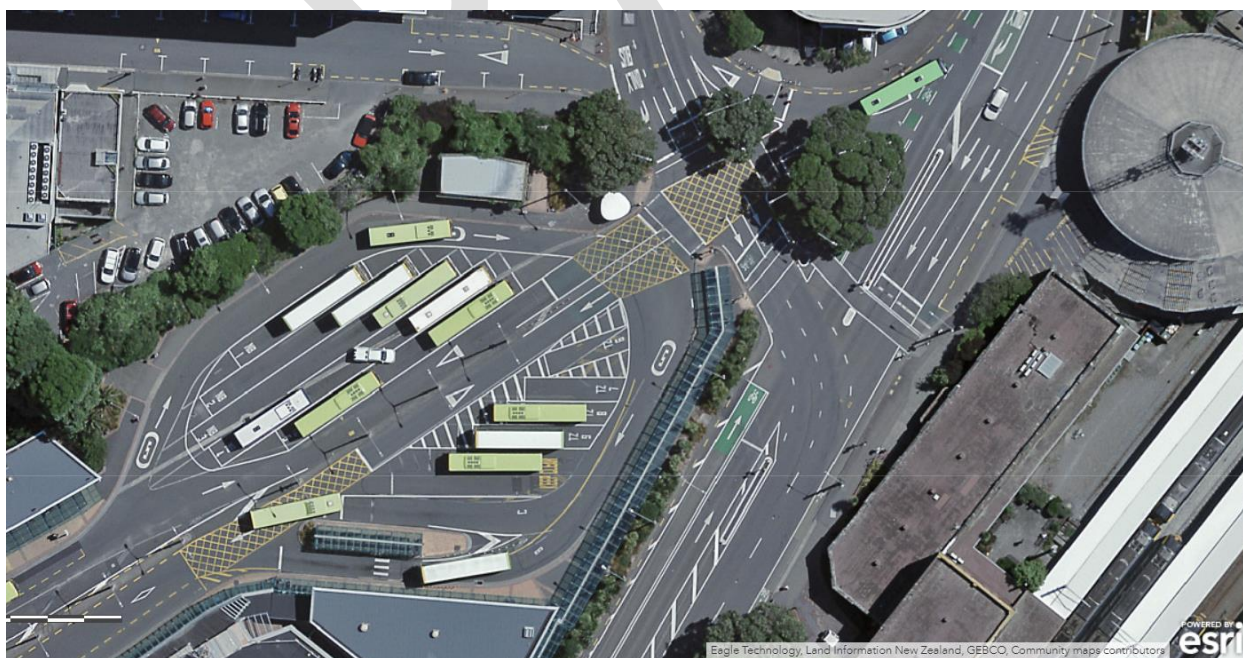
Figure 31 – Keep clear marking maintaining access to and from Wellington bus station.
