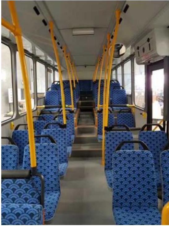
Figure 64 – Interior of a bus optimised for seating with two seats on either side of the aisle. Source: Global Bus Ventures.
