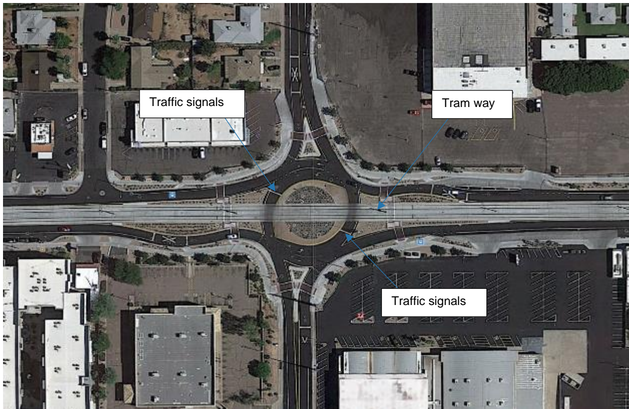
Figure 56 – Roundabout with light rail lines through the middle at the intersection of South Horne and East Main Street, Phoenix, United States. Source: Google Earth.
