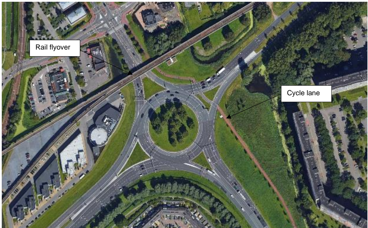
Figure 59 – Roundabout with grade separation between vehicles and trains, Capelle aan den IJssel, Rotterdam, Netherlands. Source: Google Earth.
