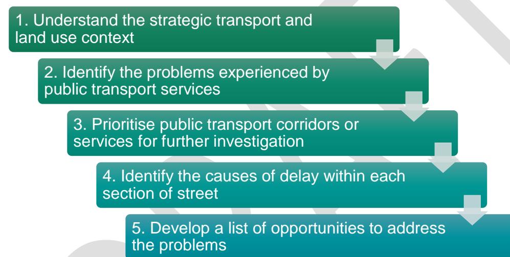
Figure 4 – High-level process for planning public transport priority projects. Source: Adapted from Austroads. 2020. On-Road Public Transport Priority Tool . Sydney.
