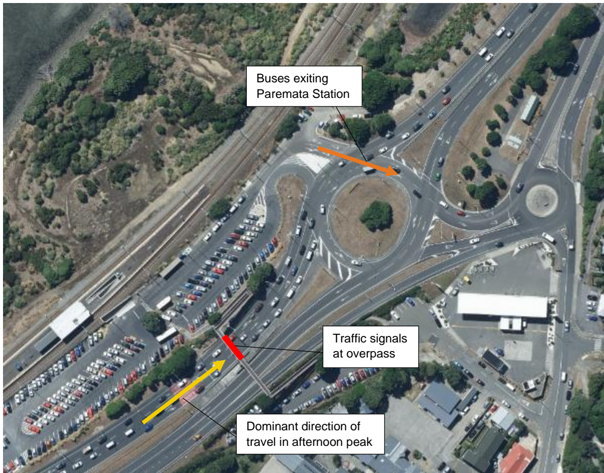
Figure 52 – Metered roundabout at intersection of State Highways 59 and 58 and Paremata Station access. Source: Porirua City Council.
