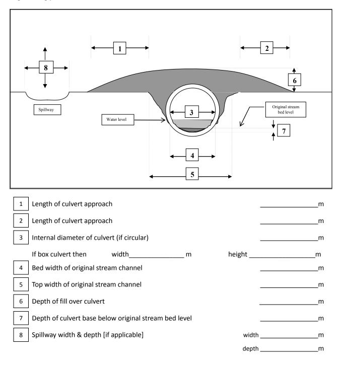
What is the proposed length of the culvert pipe?\_\_\_\_\_ m
