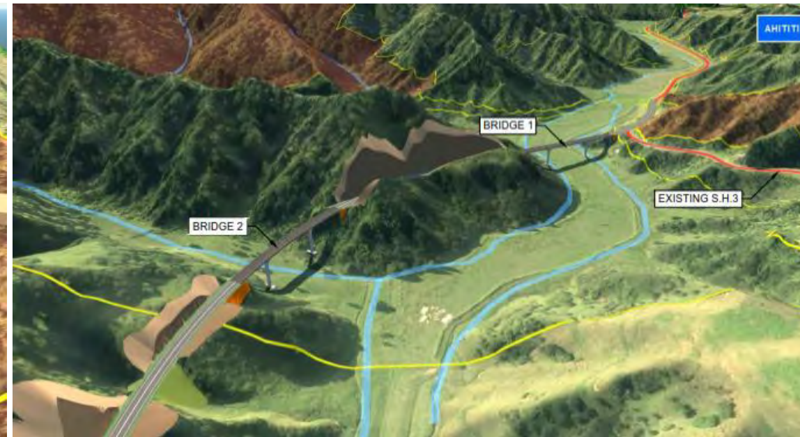
Figure 2: View along Option A towards the northern tie in to State Highway 3 (SH3)
