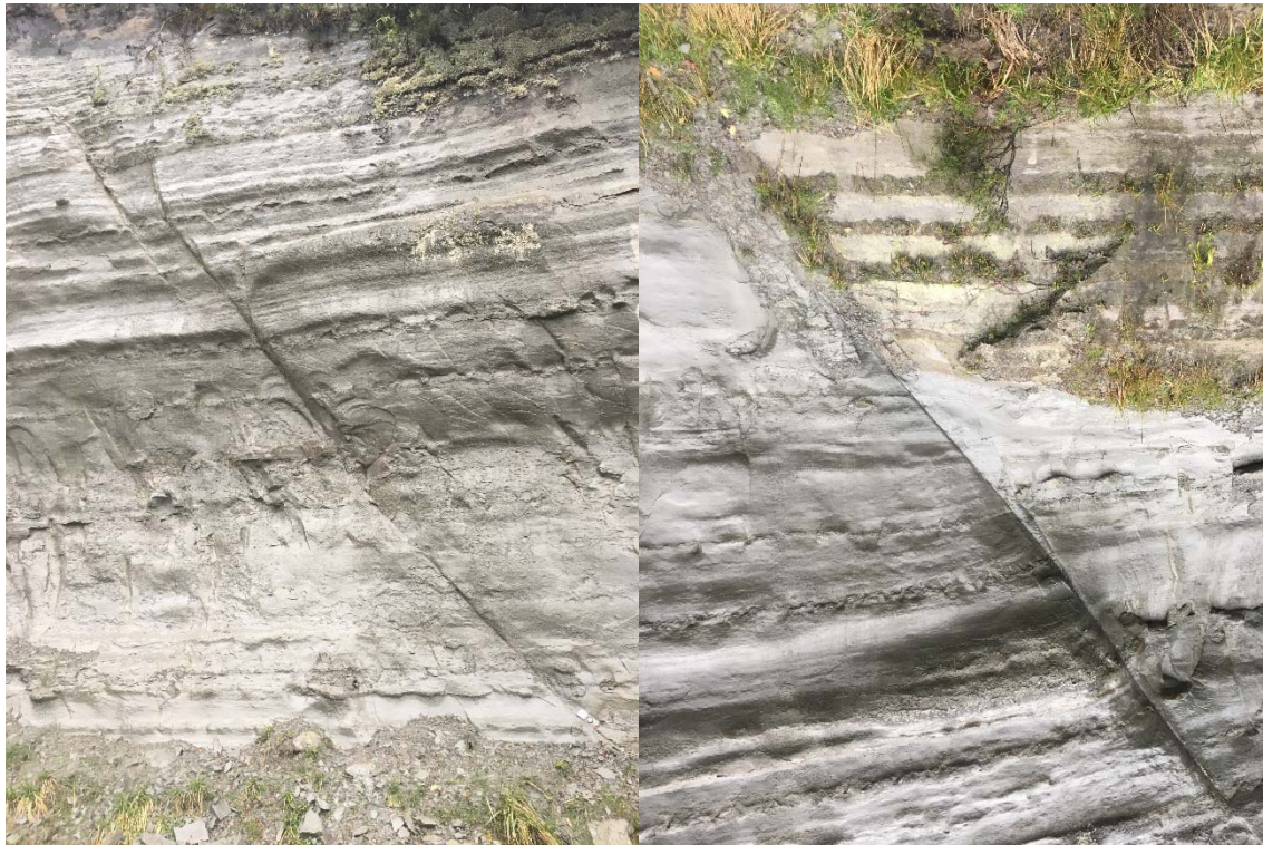
Figure 4.6 – Steeply dipping defects in the Mount Messenger Formation.
