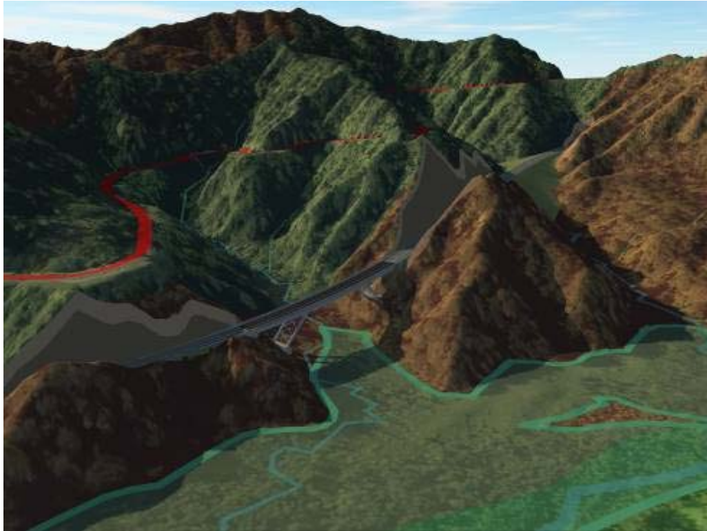
Figure 1.8 – The proposed southern tunnel approach and wetland gully bridge with rock cut approaches, with Mount Messenger on the skyline (the existing alignment is in red. The green outline area is the Mimi Valley Kahikatea wetland).
