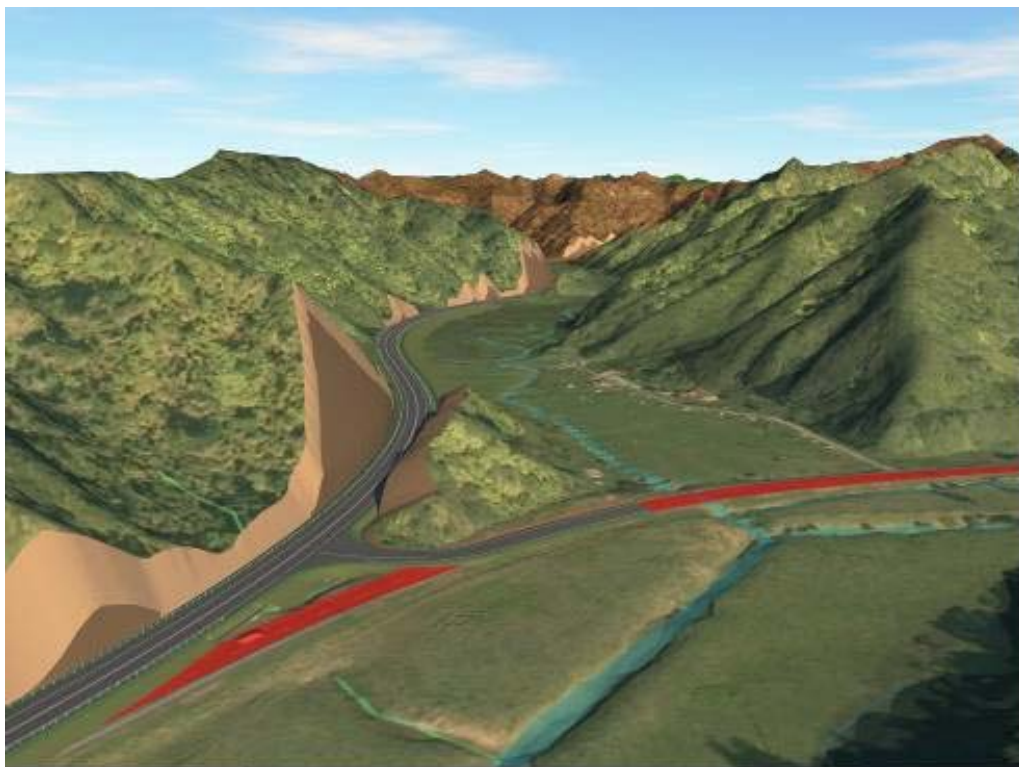
Figure 1.3 – Southerly view at the northern tie in with the existing SH3 (in red) showing toe slope rock cuts and the proposed highway to the east of the valley floor.
