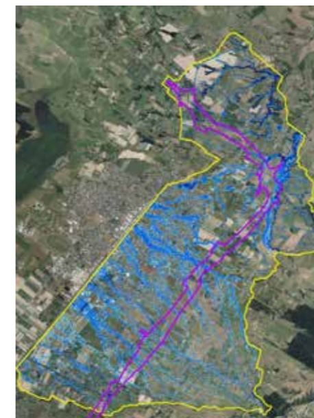
Baseline maximum modelled depths, showing 1:100 flood event in 2030 (North) [Technical Assessment - Hydrology and Flooding]
