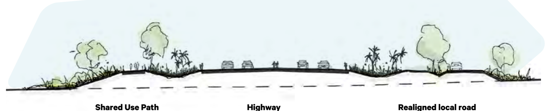
Example of 'fill' section
