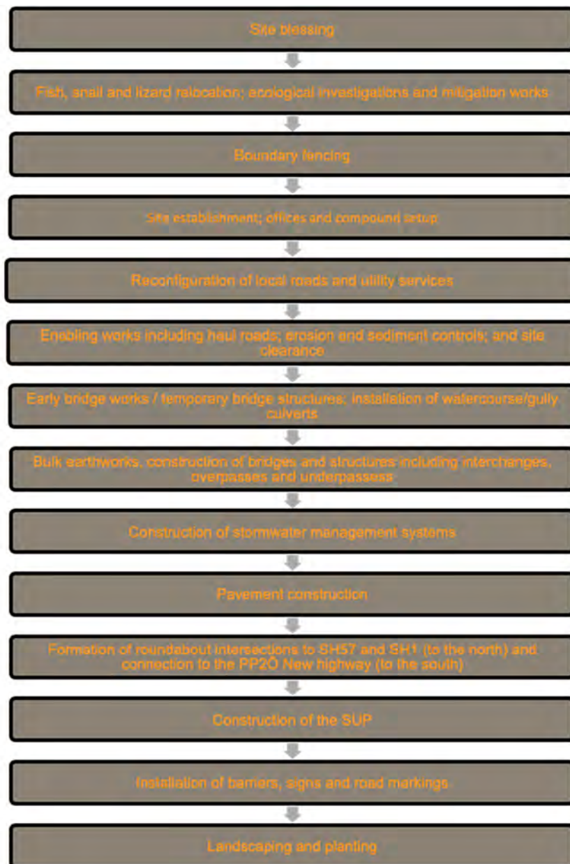
Figure 4.3.1: Indicative Construction Sequence
