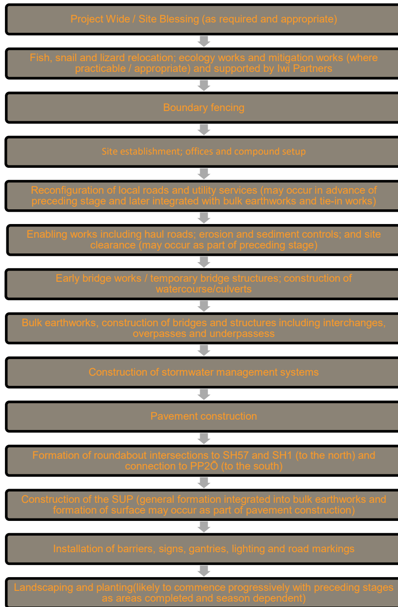
Figure 4: Possible/indicative construction sequence
