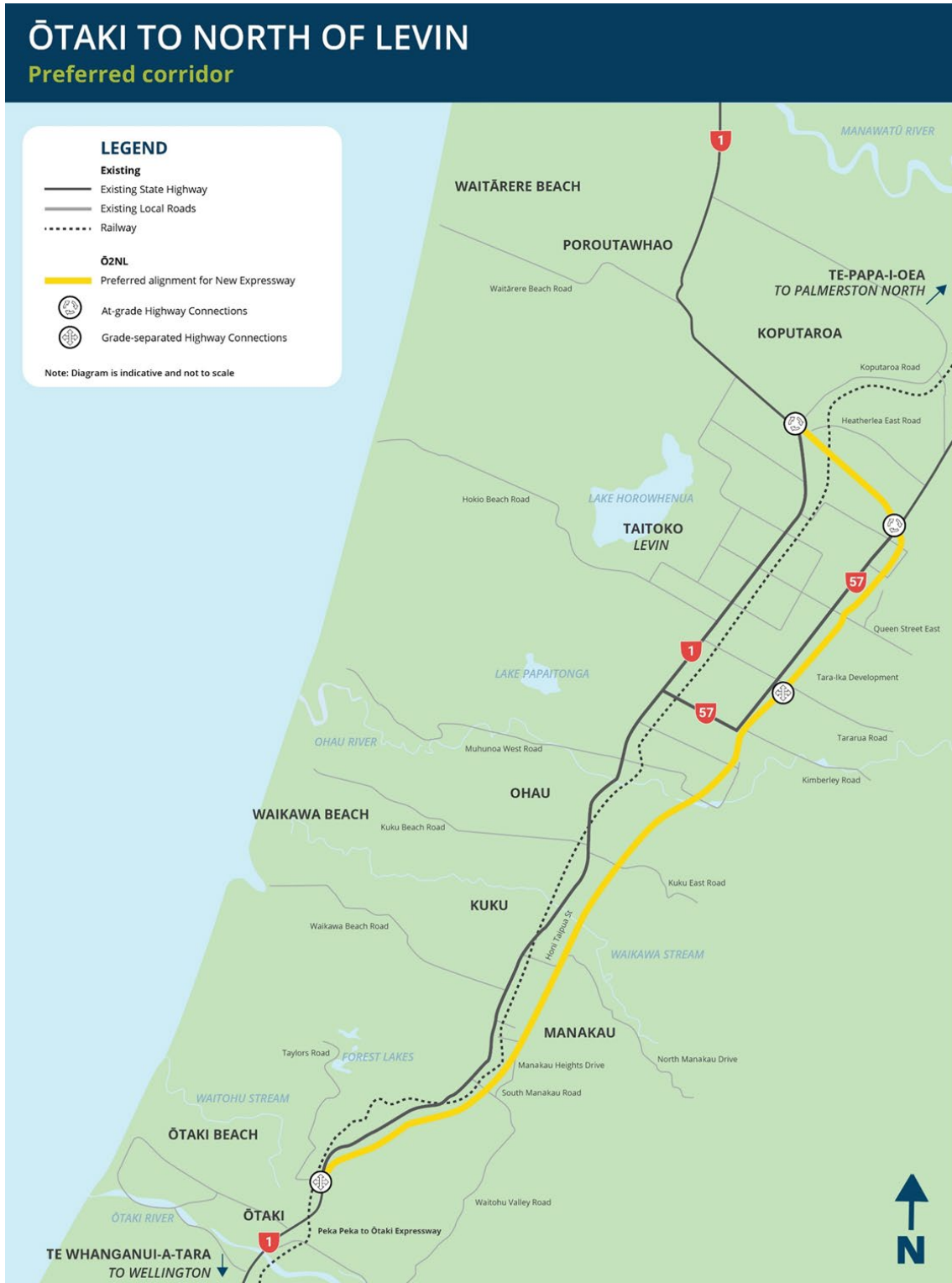
Figure 26-11 Summary of the combined southern and northern preferred corridor options for the Taylors road to north of Levin new offline highway
