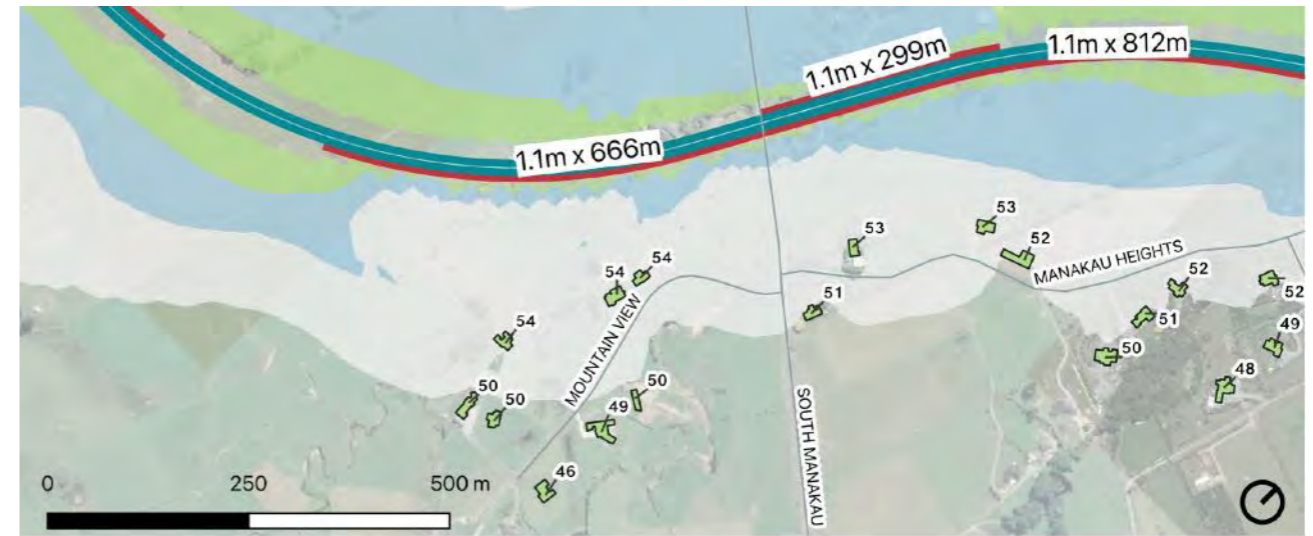
Option 2: concrete safety barrier
