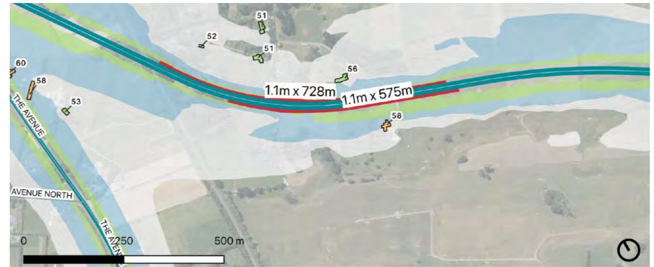
Option 2: concrete safety barrier
