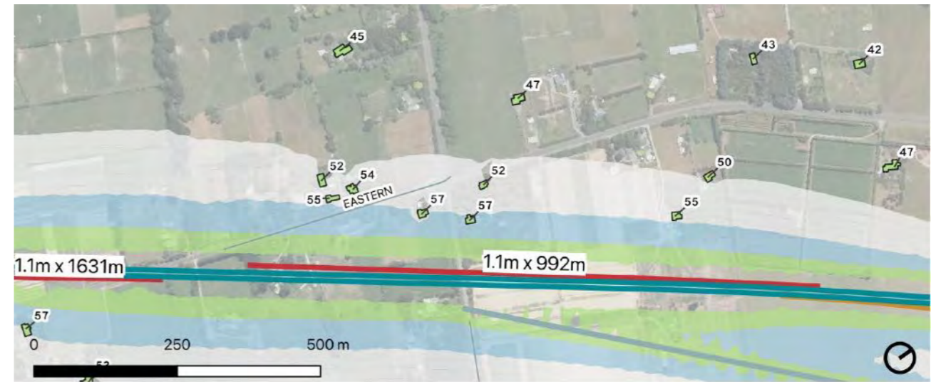
Option 2: concrete safety barrier
