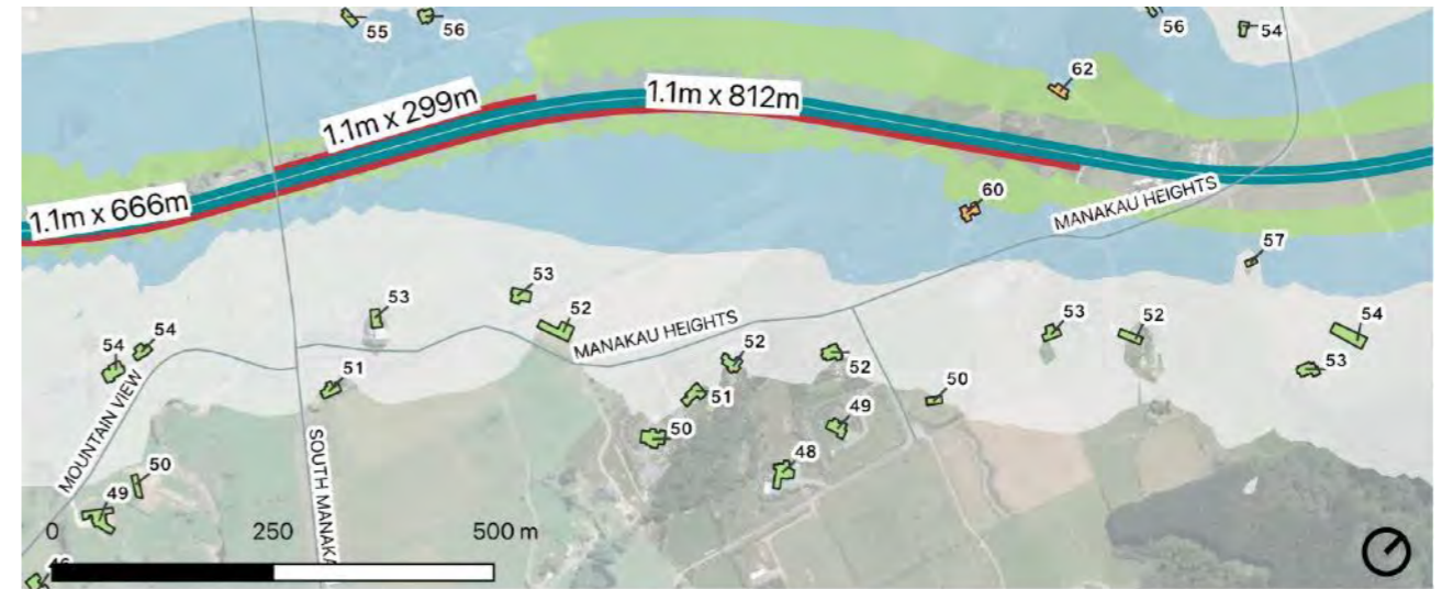
Option 2: concrete safety barrier
