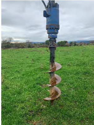
Left image: Clean drill before sampling ORSL1
