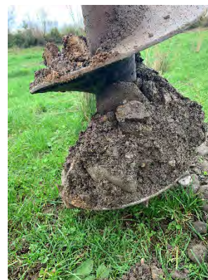
Left image: Site ORSL_1 at 0.4 m depth. The soil is similar in colour throughout.
