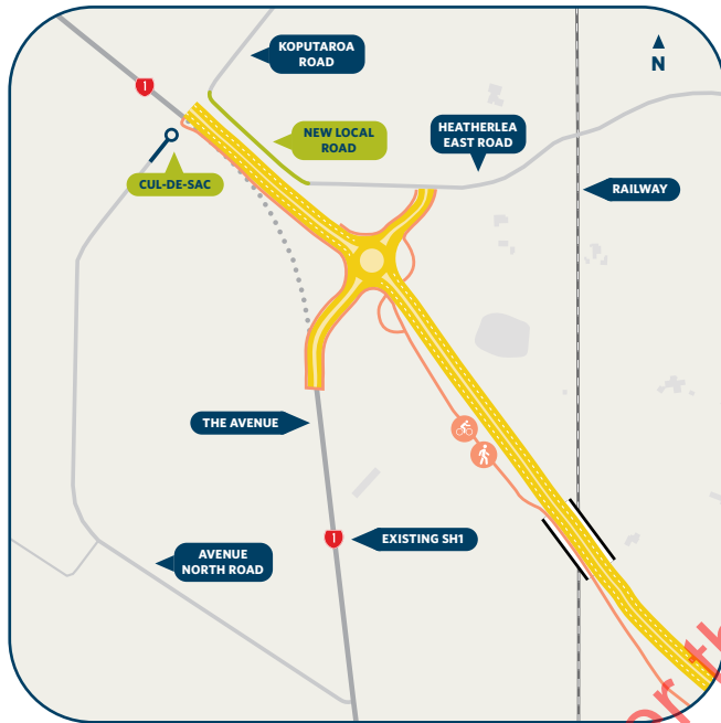
New dual-lane roundabout to connect the new highway to the existing SH1 near Heatherlea East Road. Avenue North Road will connect to the existing SH1 in the south and will end in a cul-de-sac at the northern end.
