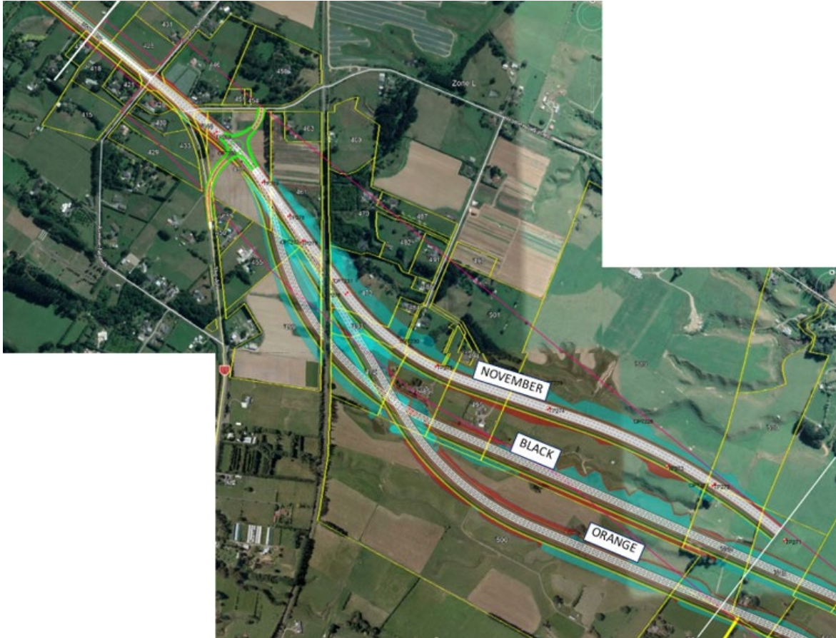
Figure 16: New (November 2020) alignment and the original preferred alignments (Orange and Black) for Zone L
