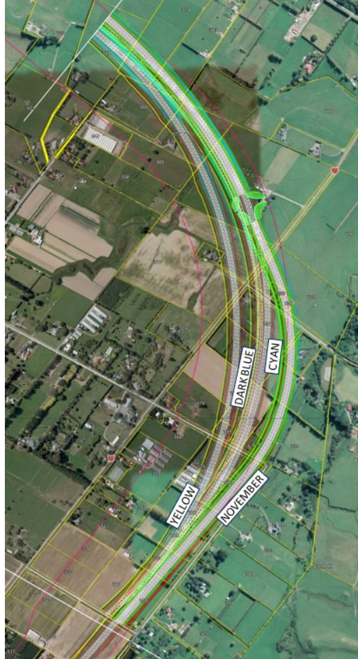
Figure 15: New (November 2020) alignment and the original preferred alignments (Yellow and Dark Blue) for Zone K
