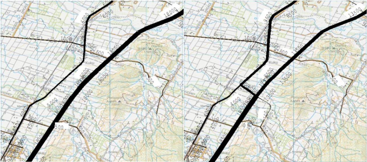
Figure 3-1: A comparison between traffic flows for scenario 2 and scenario 4 (with and without South Kuku interchange)
