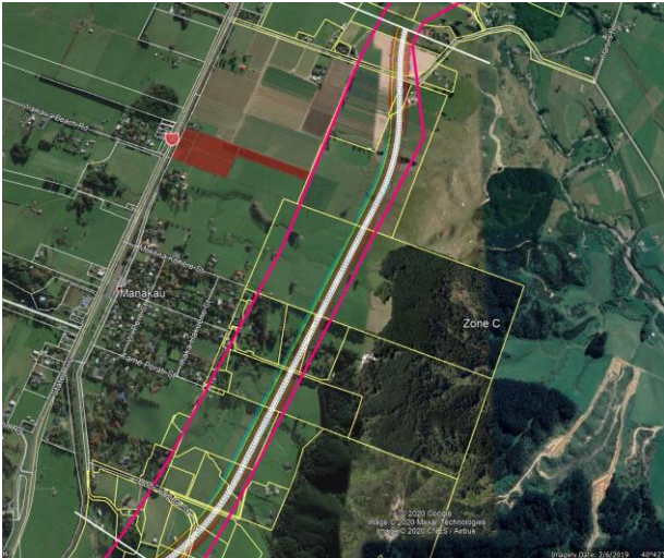
Figure 6 – Draft preferred White alignment option for Zone C (as identified in the Draft MCA Report)
