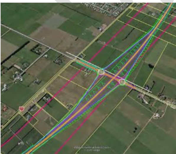
Figure 18 – An example of a full diamond shaped interchange at Tararua Road
