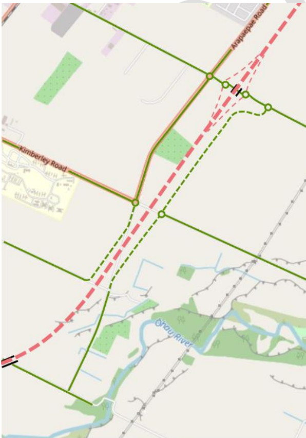
Figure 26 – Option 2: Connections at Tararua and Muhunua East Roads (no connection at Kimberley Road)
