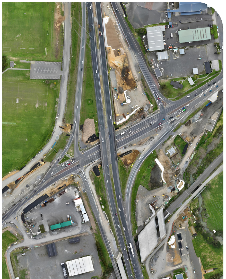
Earthworks are underway in the northeastern gore at Drury Interchange ahead of piling works for the new motorway bridge across Great South Road, scheduled to begin in late 2025/early 2026.
