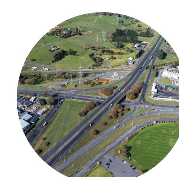
Interchange improvements at Drury, enabling rail electrification, future-proofing for additional rail lines, and improved access for overdimension vehicles.
