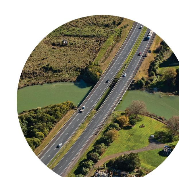
Bridges at Otuuwairoa (Slippery Creek) and Ngaakooroa Streams will be raised to provide resilience for climate change. Drury interchange and a proposed new interchange south of Drury, will be designed to allow for 100-year flood predictions.
