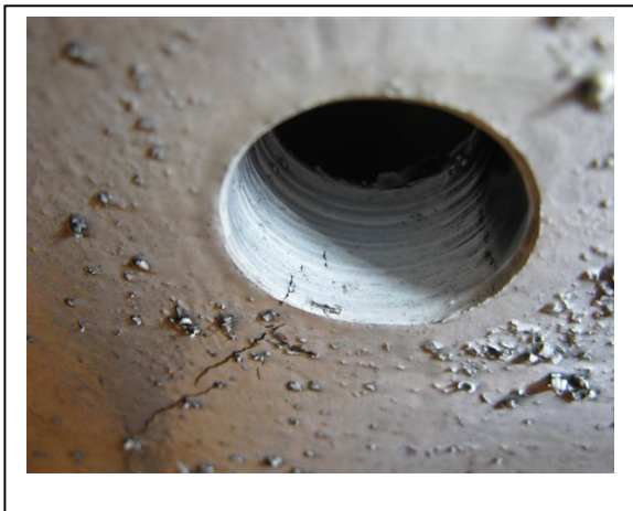
Plate Sample showing the delaminated plate acting as a natural crack arrestor
