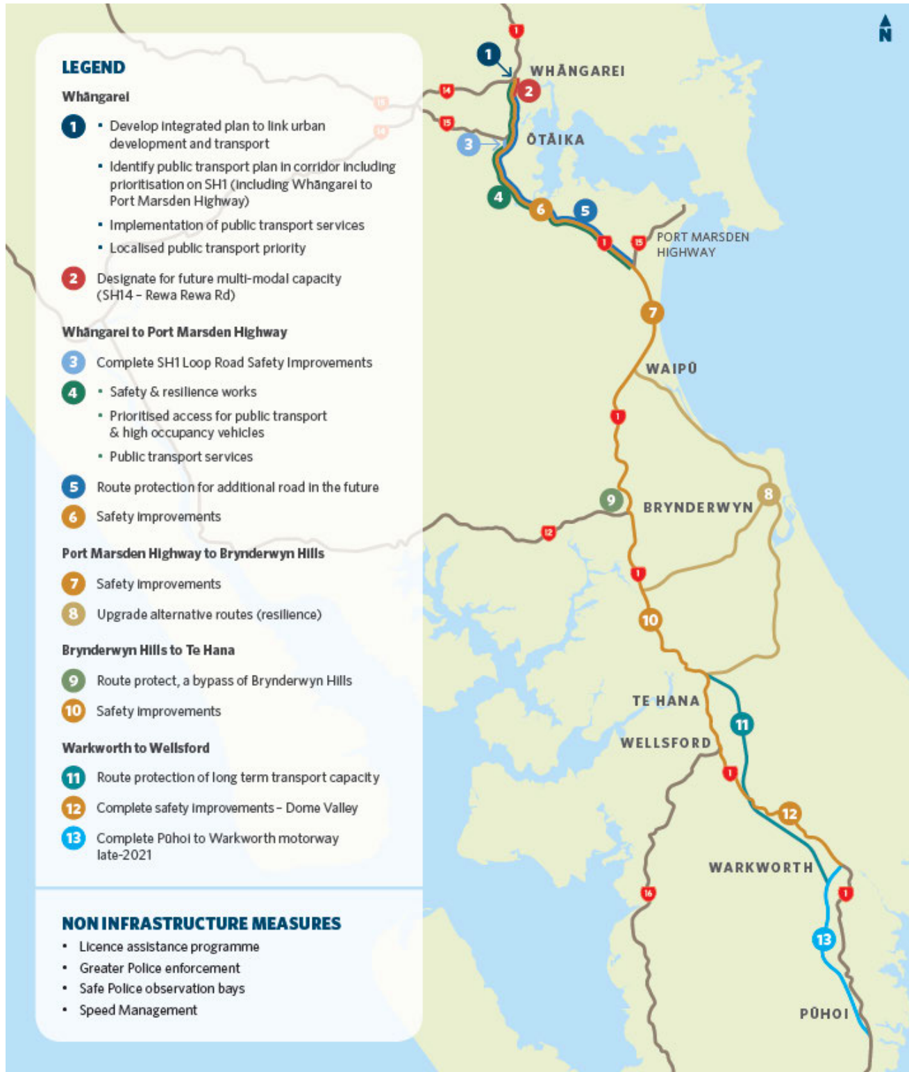
Figure 9 – SH1 Whāngārei to Te Hana corridor revised programme interventions (as part of wider Whāngārei to Warkworth recommended programme)
