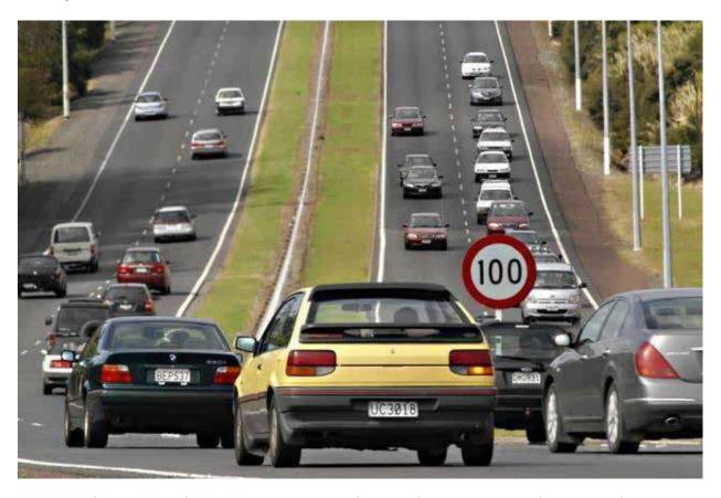
**Issue**: Median grass – dangerous to mow, weed-eat and/or spray around wire rope barriers. Issue leads to lane closures and traffic congestion. Light pole maintenance is also an operational hazard.
