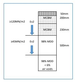
The following construction performance criteria are hence specified for the supporting pavement layers under the Hi-Lab:
