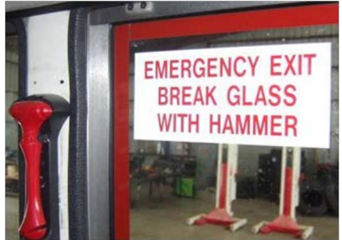
Emergency exit sign less than 75mm high displayed inside with a 20 mm wide contrasting band around.
