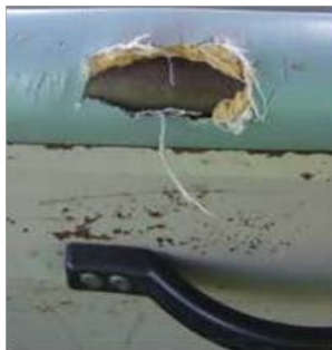
Damaged energy-absorbent material at seat backrest.
