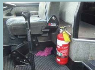
Fire extinguisher located by the driver's seat is seen by passengers when boarding.
