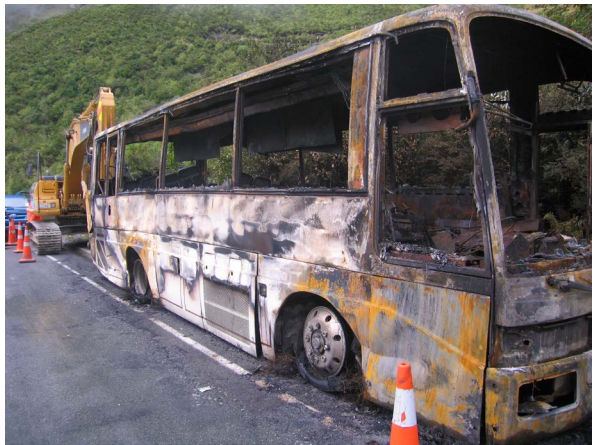
Fire started in the engine compartment.
