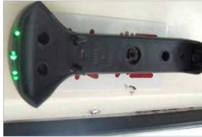
Remove device (hammer) to ensure alarm operation.
