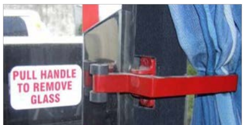
Two handles fitted on either side to pop the glass out.
