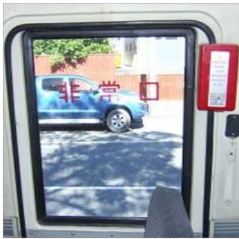
Unmarked dedicated emergency exit.
