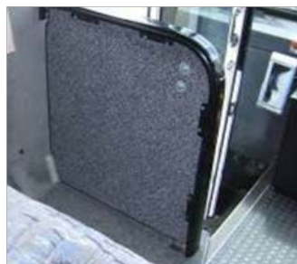
Panel fitted on the left hand side of the stairwell in front of the seat.
