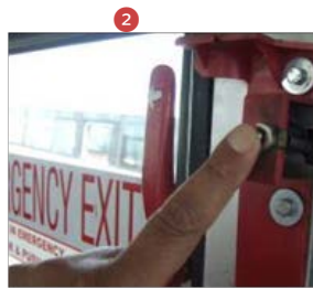
Emergency exit sign with (75mm high), glass breaking device (hammer) and instructions affixed inside.
