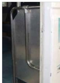
Guardrail (and panel) located between the stairwell and the front of the seat.
