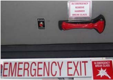
Emergency exit sign with (75mm high), glass breaking device (hammer) and instructions affixed inside.
