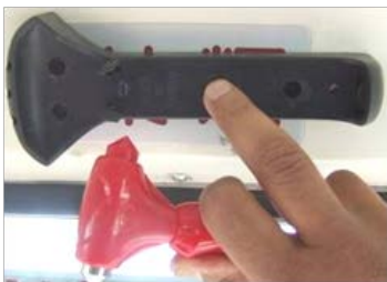
When the button is pushed-in, the alarm must stop.
