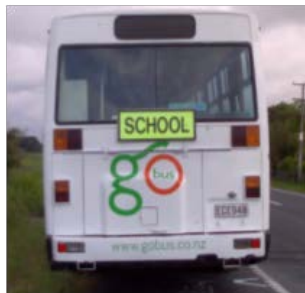
Rear sign above 1.5m from the ground.
