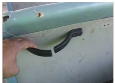
Damaged and missing handholds.
