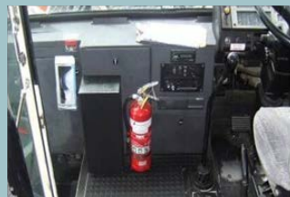
Fire extinguisher located between the front door and the driver's seat visible to passengers.
