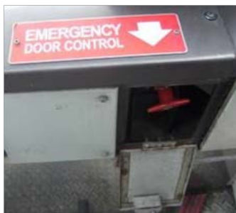
The red knob releases door operating pressure to open door from inside (and outside) in an emergency.
