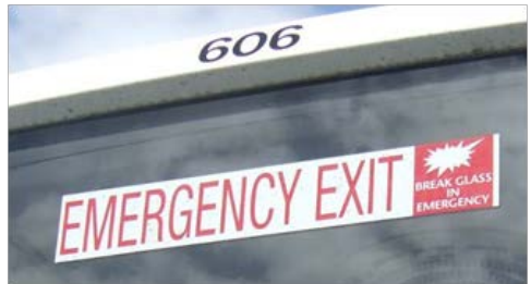
Emergency exit sign with 75mm high letters (must be both inside and outside). No contrasting band required. In this instance, glass breaking instructions incorporated.
