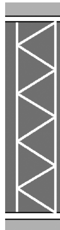
Figure 15.12 – Reflective 'zigzag' marking on platform approach, lines 150mm wide
