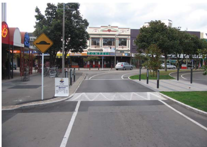
Photo 6.23 – Pedestrian platform, Palmerston North (Photo: Glenn Connolly)
