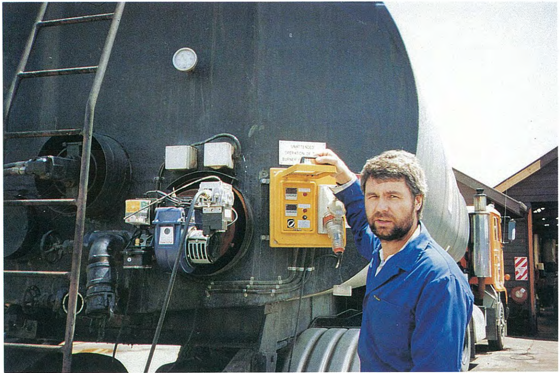
Burner and Thermostatic Control Box.
