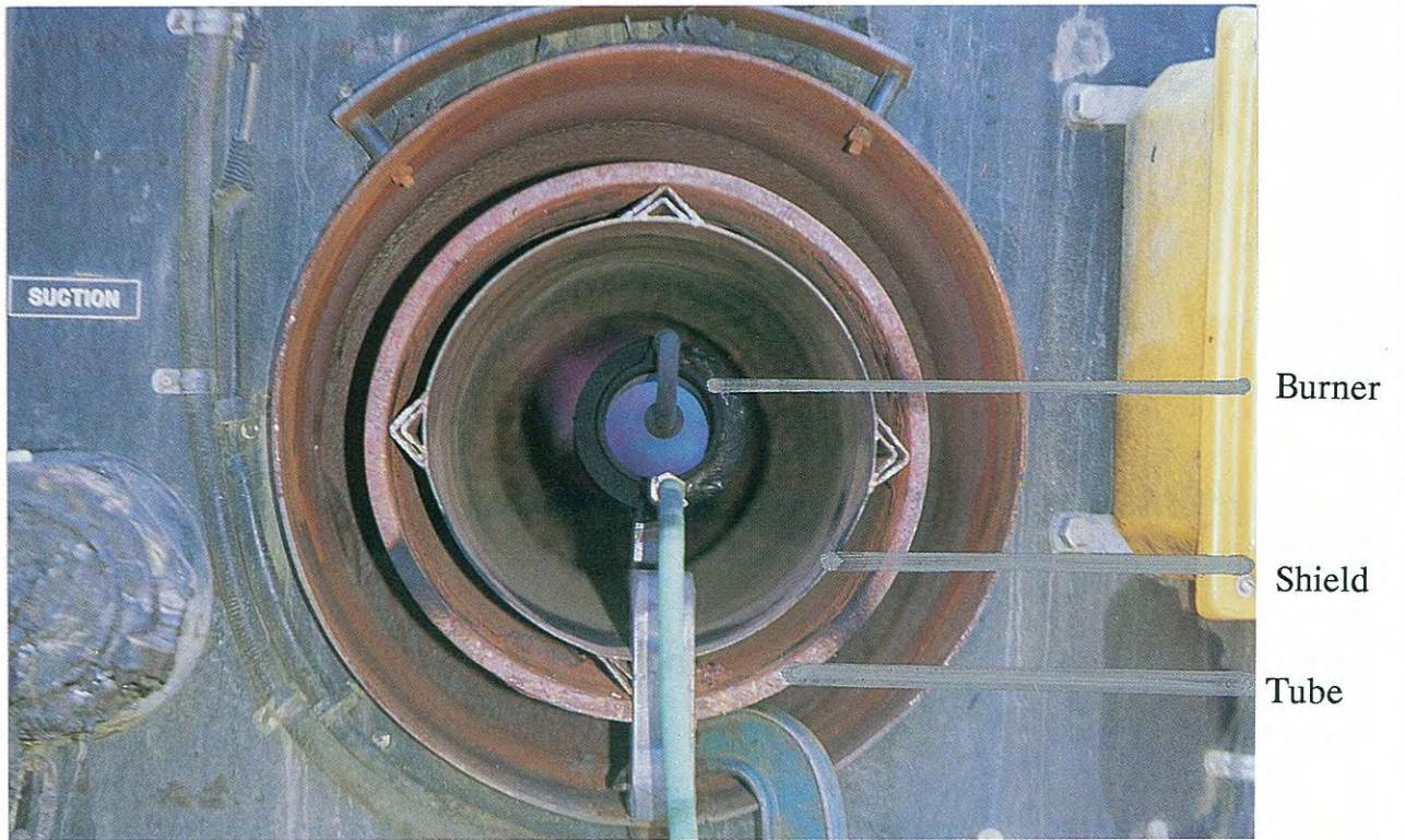
Mattheus burner inside flame tube, showing relative diameters of shield and tube.
