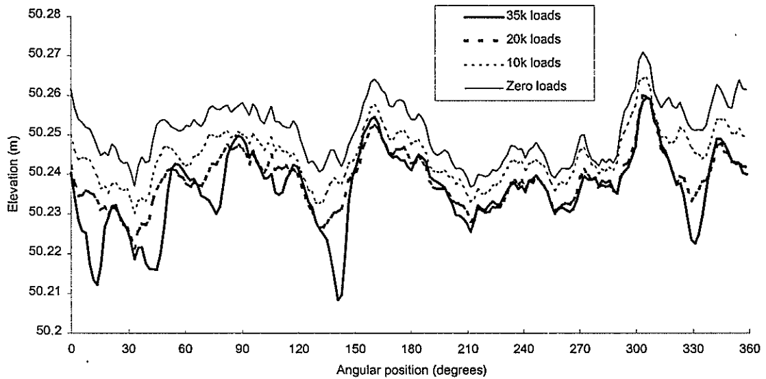
Figure 2.5 Longitudinal profiles for inner wheel path.
