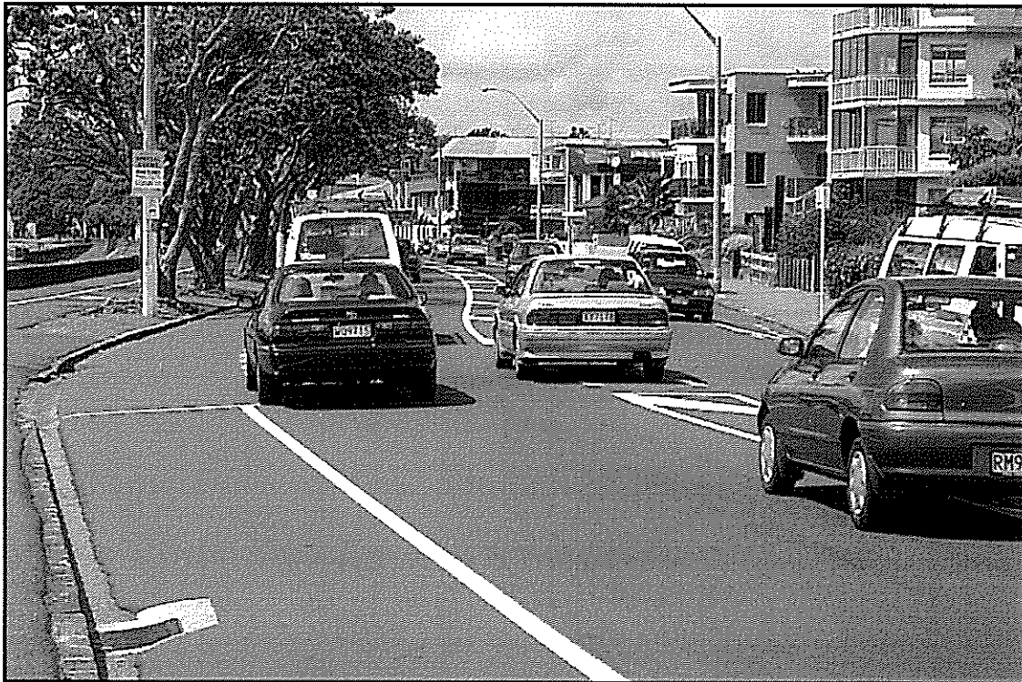
Figure 4.3 Safe operation of narrow flush medians.
