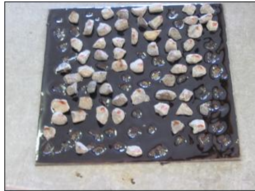
Figure 6.2 Vialit Plate after testing (53% retained).
