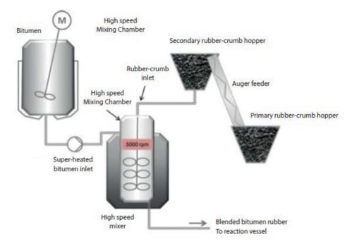
Once the CRB is produced then it goes straight to a specialised sprayer (field blended) that can cope with the high viscosity of the CRB. For fixed plant blended products, the CRB goes into a storage tank but is used within the maximum storage time. Note that in the USA, terminal blend can mean 'fully digested' crumb rubber binder. However, this would have vastly different rheological properties, as described earlier.
