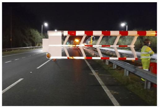
Figure 2.26 SwiftGate remotely deploying gate (reprinted from Fossdyke, 2022)
