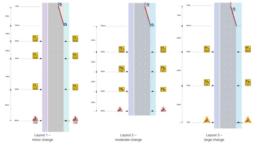
Figure 2.15 Alternative layouts for single-lane closures on dual carriageways (reprinted from Wood et al., 2011, pp. 7–9)
