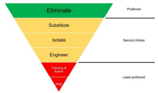
Figure 2.9 Austroads' hierarchy of controls (reprinted from Austroads, 2021a, p. 15)
