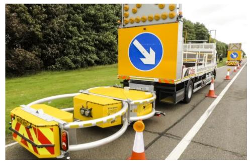
Figure 2.32 Colas autonomous IPV in action (reprinted from Colas, 2017)
