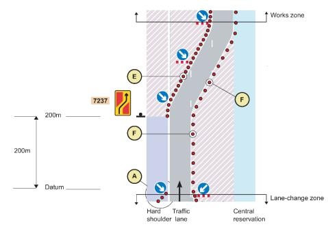
To install the 'facing wall of cones', workers must enter the only remaining open lane in the face of oncoming traffic, utilising what gaps they can find in the stream – a risky activity. If the work zone is left with the wall incomplete due to the low traffic window of opportunity passing, risk to road users is heightened due to the incomplete lead-in zone.
