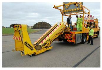
Figure 2.30 Conemaster cone deposit and retrieval system (reprinted from Highways Agency, n.d., p. 3)
