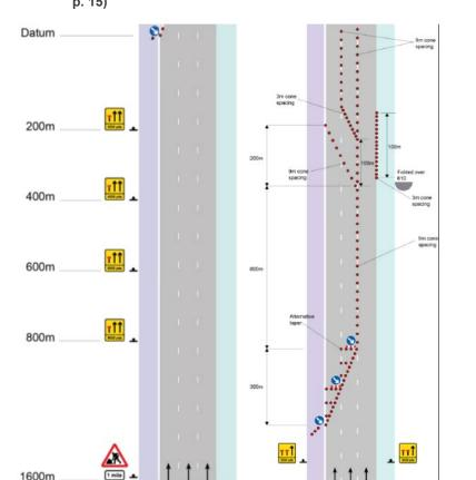
Figure 2.19 TTM layout used during trials, consisting of offside signs removal advance signing (left) and 'alternative' taper, longitudinal coning, and lead-in zone (right) (reprinted from Palmer et al., 2015, p. 15)
