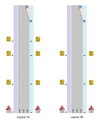
Figure 2.16 Two alternative lane closure layouts trialled (reprinted from Wood et al., 2011, p. 14)
