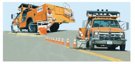
Figure 2.29 AHMCT cone placement and retrieval vehicle (reprinted from AHMCT, n.d.)
