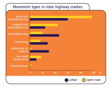
Typically these crashes were a single vehicle crash, with loss of control on a right-hand or left-hand curve.
