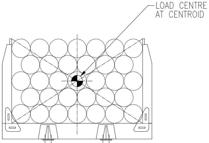
*Figure 1 Determination of the load centre position*
