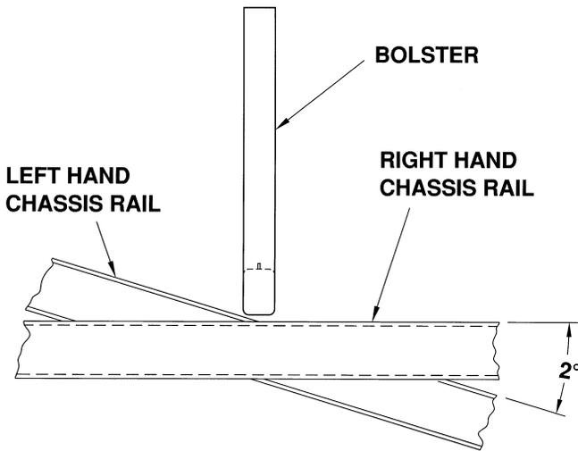
*Figure 5 Torsionally Independent Bolster Attachments:
