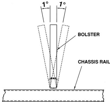
*Figure 6 Angular displacement requirement for sliding and resilient bolster attachments (not to scale)*
