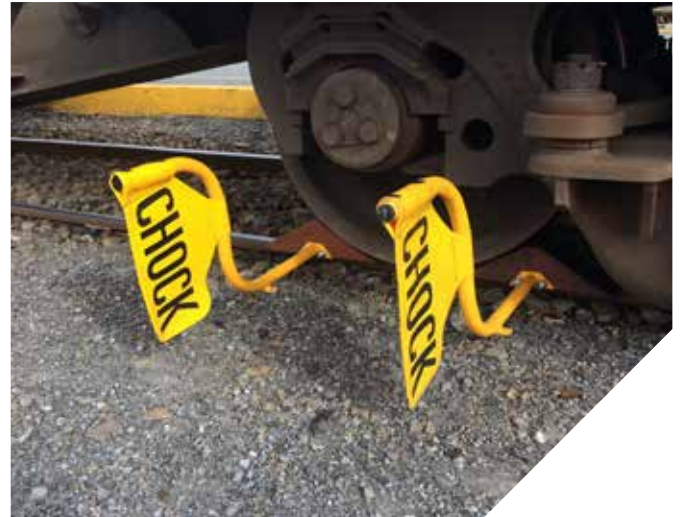
Rail vehicle stabilised to KiwiRail's new chocking code. Photo: KiwiRail.
