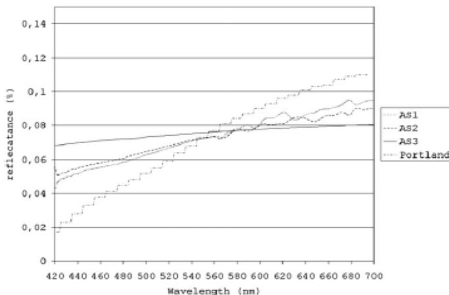
Figure 25: Spectral reflectance of four surfaces from Falchi et al, 2011<sup>12</sup>.
