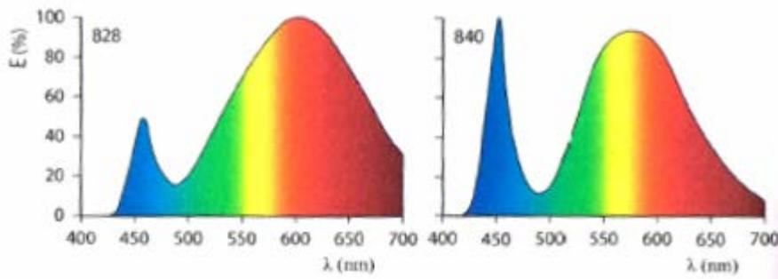
Figure 8: Spectral Power Distributions of two LED sources: Leftmost 2800K, rightmost 4000K
