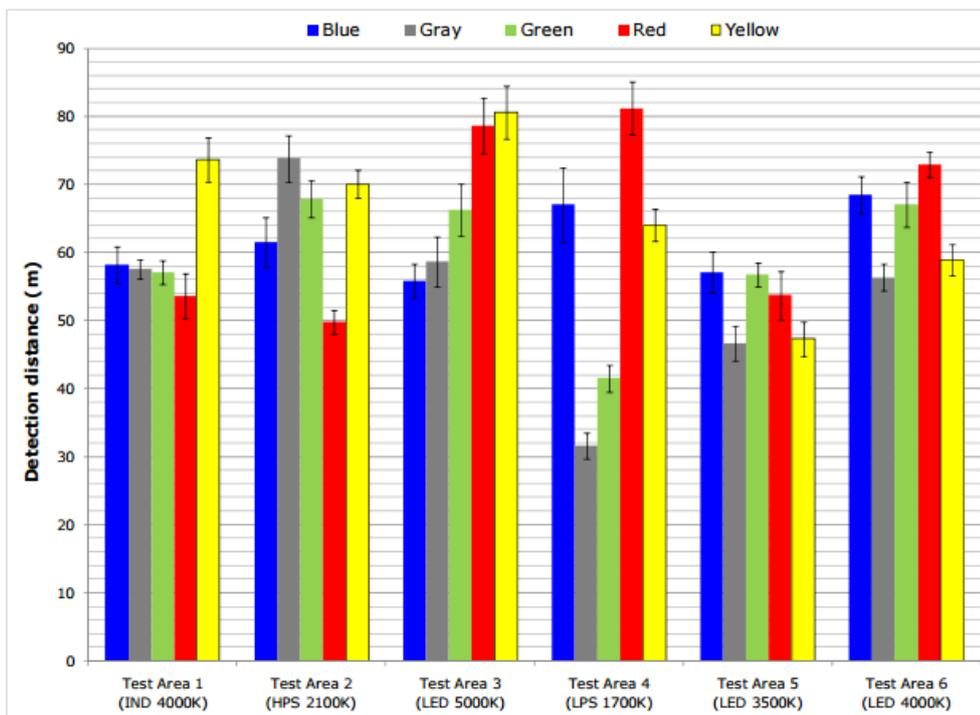
**Figure 15: Detection distances by light source and colour-San Jose Wet Surface**
