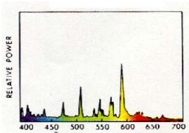
Figure 6: Metal halide spectral power distribution chart
