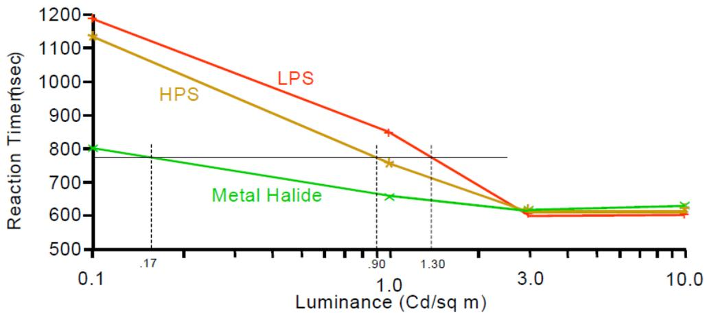
Figure 10: Reaction time versus luminance for HPS, LPS (both yellow) and metal halide (white)
