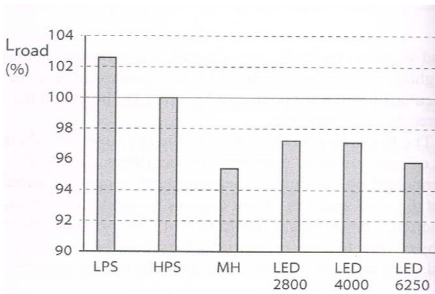
Figure 26: Surface luminance for an asphalt surface and various light sources relative to HPS.
