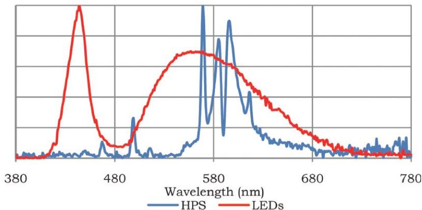
**Figure 20: Spectra of the HPS and LED light sources used by Fusheng et al.**
