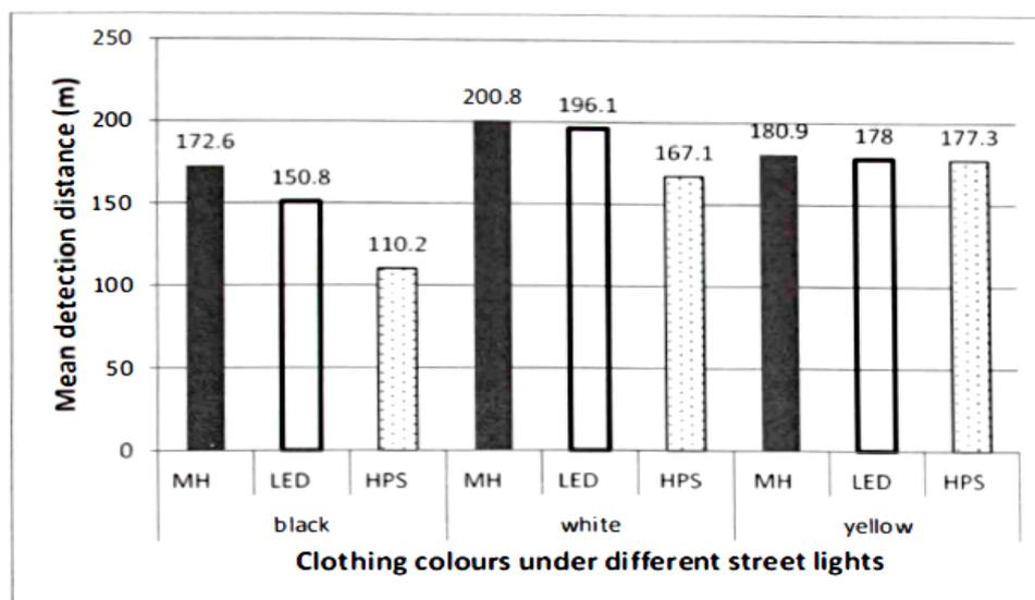
Figure 12: Mean pedestrian detection distances by light source and clothing colour.
