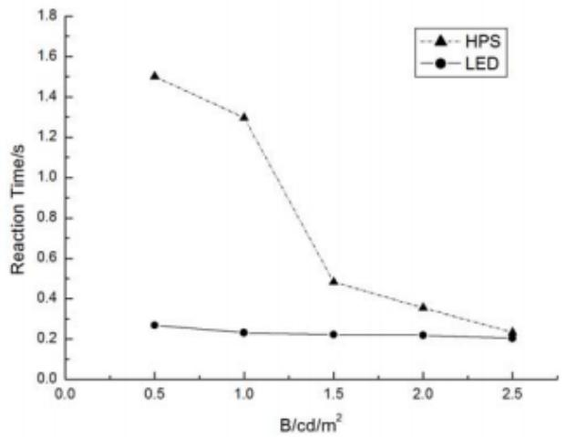
**Figure 13: Curve relating reaction time to luminance using HPS and LED**
