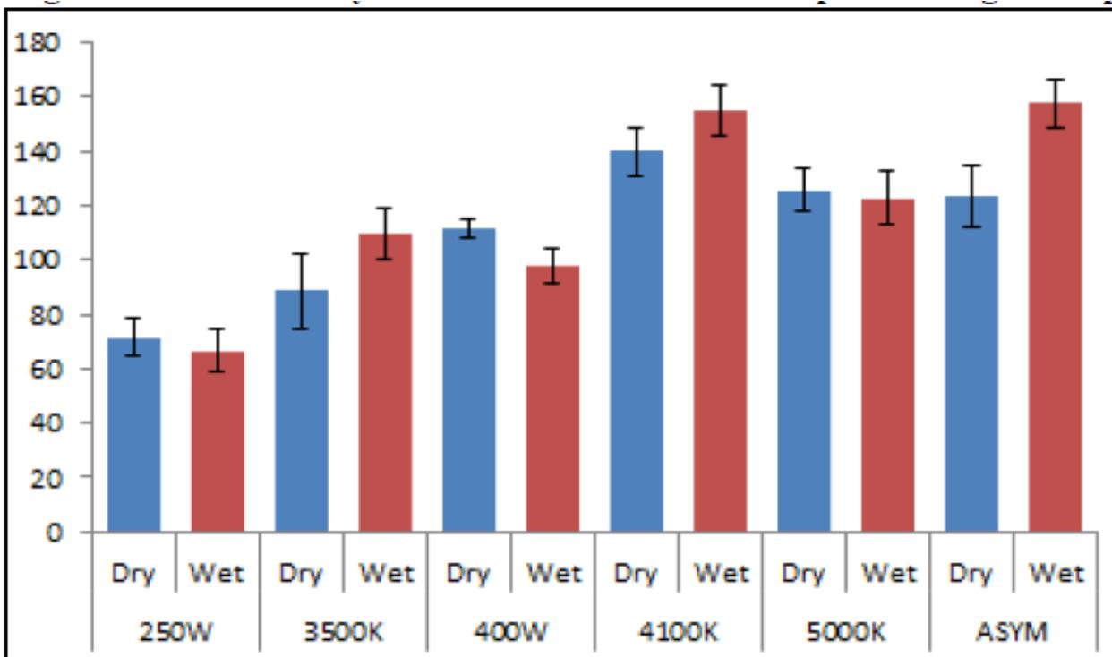
Figure 17: Detection distances for wet and dry conditions for undimmed luminaires -Seattle.
