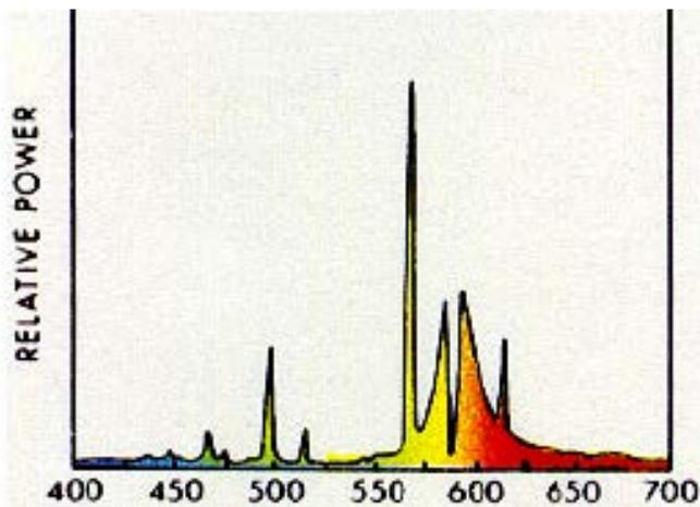
Figure 5: HPS spectral power distribution chart
