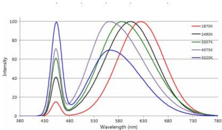
Figure 30: Spectra of LEDs used by Jin et al, 2015
