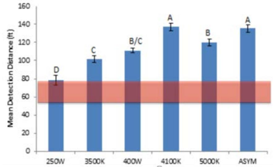
**Figure 19: Detection distance comparison of Seattle Luminaires-using wet and dry road data**
