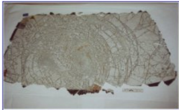
Photograph 12 Reassembled laminated screen
