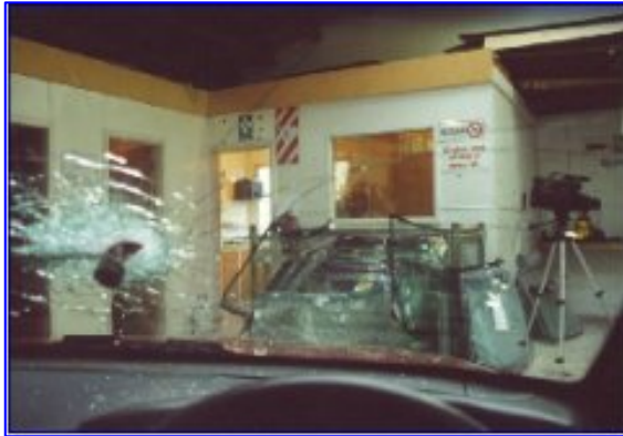
Photograph 11 Damaged laminated screen.
