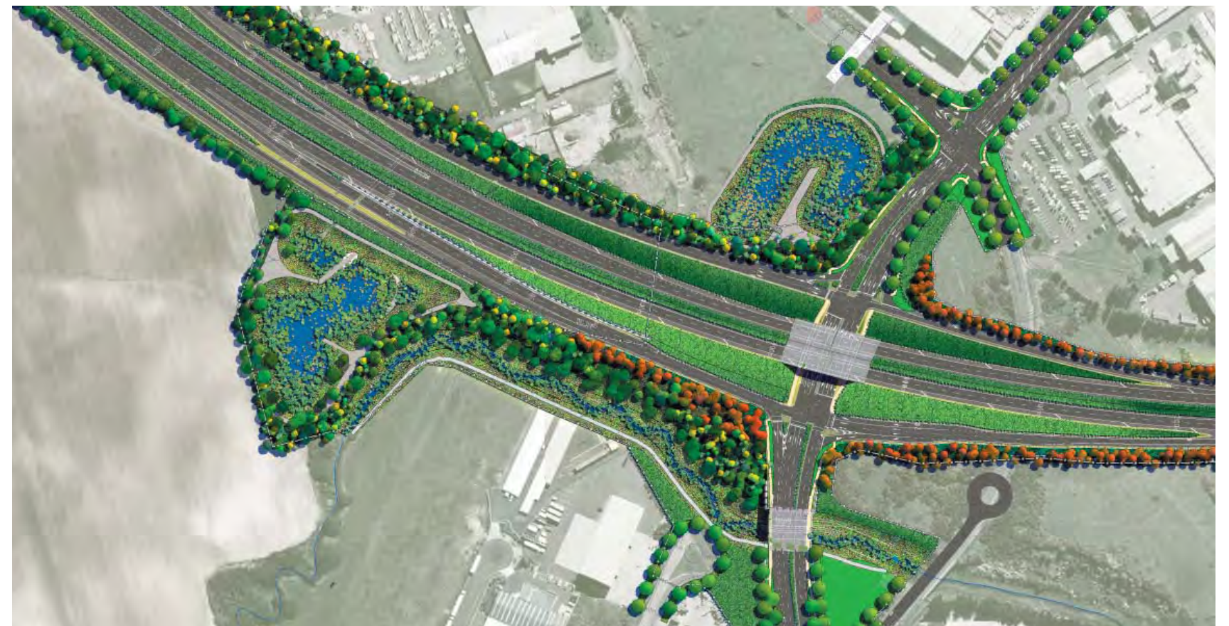
Figure 9.8 - Puhinui Stream diversion and stormwater pond.
