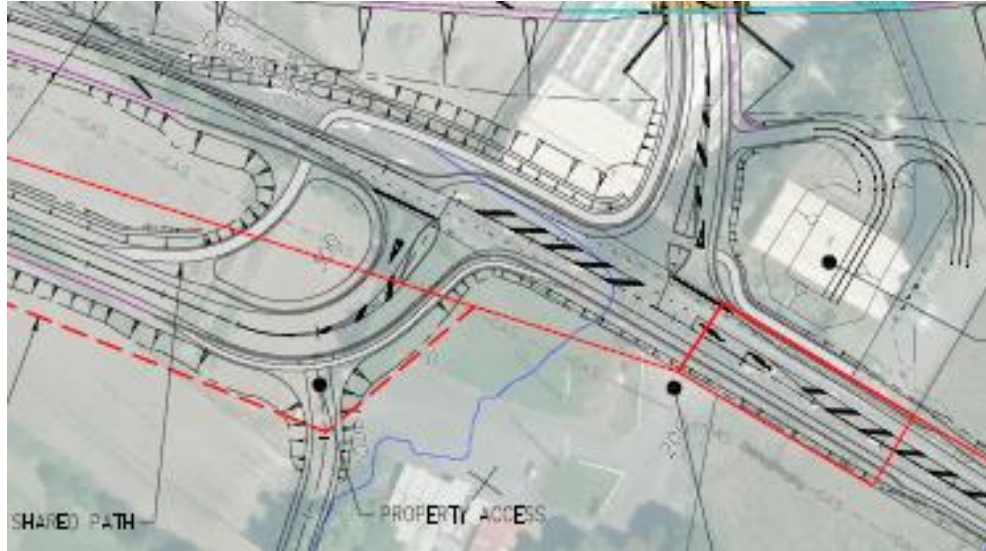
Figure 2: Staggered intersection at Coast Road/Paekakariki northbound on-ramp
