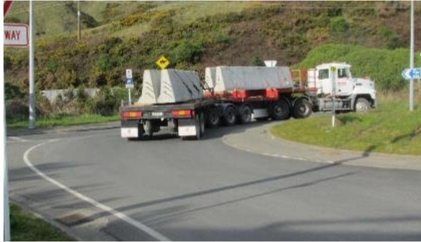
Figure 3: Large truck and trailer unit negotiating roundabout at MacKays
